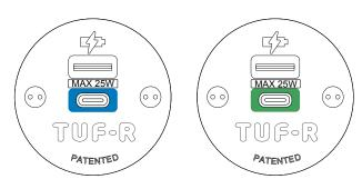
Both TUF 25W and TUF HP have short circuit protection that is self resetting.
